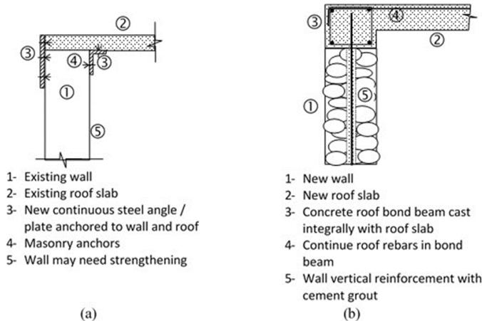
Figure 2: Improving connectivity of roof with walls. (a) Existing construction, (b) New construction
