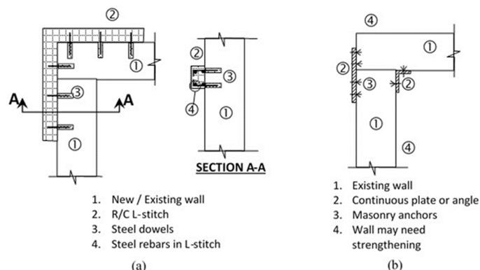
Figure 3: Improving connection between walls. (a) L-stitch in new construction, (b) Continuity element for existing construction
