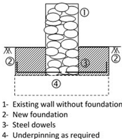
Figure 4: Detail of foundation strengthening in an existing structure
