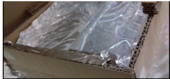
Figure 7 Plastic bag filled with water that act as roof pond
