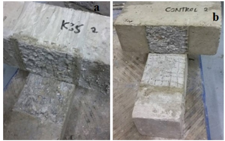
Figure 9 Interface failure mode of tensile test sample (a) KFCC (b) PC
