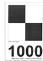
Figure 4 Example of black and white (B&W) target used with TLS ( https://www.point3d.us.com/product-page/tuff-targets-100-pack )
