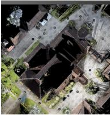
Figure 6 Positioning of Leica Terrestrial Laser Scanner P16 during scanning (Authors' work)
