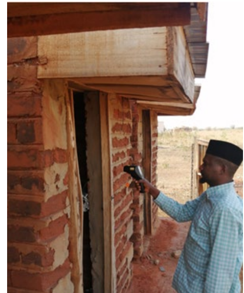
Figure 10. Testo Infrared thermometer surface temperature monitoring
